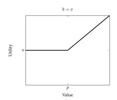
Figure 3: Utility as a function of value, when bidding truthfully, assuming the highest other-agent bid is fixed at *p*.
