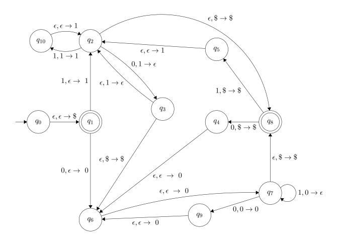
All undrawn transitions are assumed to go to the sink state (it'll turn out that no input string halts in the sink state by the way that we control the stack, but we must include it anyways).
