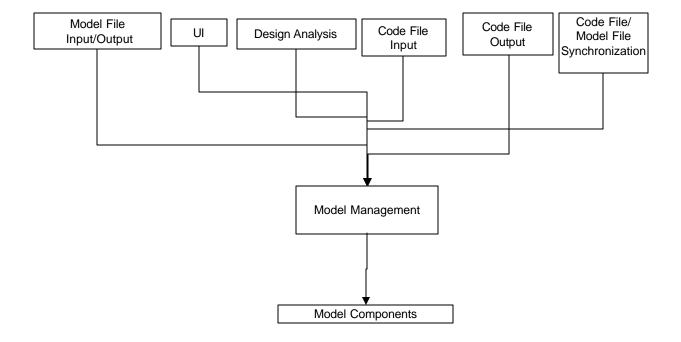
Three levels of the system are presented in fig. 1 in relation of *dependency*. At the base are the *model components*. The inheritance diagram for these classes is displayed in fig. 2. These components contain information about the visual presentation and layout as well as *functional* information. For example, a *class* object contains the screen coordinates for display as well as links to all of the *connections* and *groups* it is associated with.
