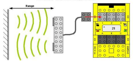
Attach the Ultrasonic Range Sensor as shown. The sensor port should be set to light sensor mode. With the Lego firm were loaded, use the View button to select the port and observe the value displayed. The distance to the target surface is the range as follows;
