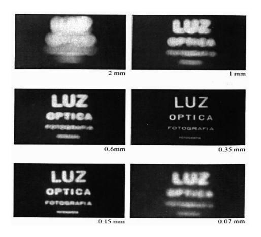
Light diffracts as wavelength of aperture equals wavelength of light
