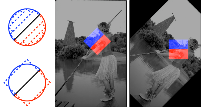
Fig. 21. Efficient computation of the oriented gradient of histograms. Left: The two half-discs of interest can be approximated arbitrarily well by a series of rectangular boxes. We found a single box of equal area to the half-disc to be a sufficient approximation. Middle: Replacing the circular disc of Figure 4 with the approximation reduces the problem to computing the histograms within rectangular regions. Right: Instead of rotating the rectangles, rotate the image and use the integral image trick to compute the histograms efficiently. Rotate the final result to map it back to the original coordinate frame.
