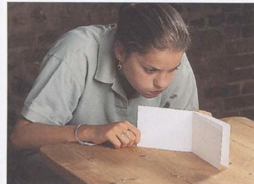
Bernoulli's principle is demonstrated by blowing between two sheets of paper.
