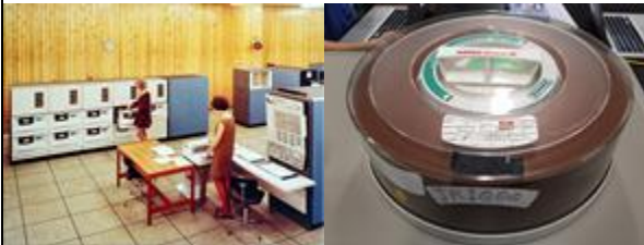
IBM System 360/65 with 2314 disk unit; 8x25MB = 200 Mbytes (late 1960's)
