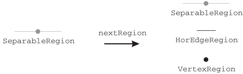
Figure 9: The possible objects returned by method nextRegion(DiscrimResult) when invoked by a SeparableRegion modeling the recursive decomposition of a horizontal subchain.
