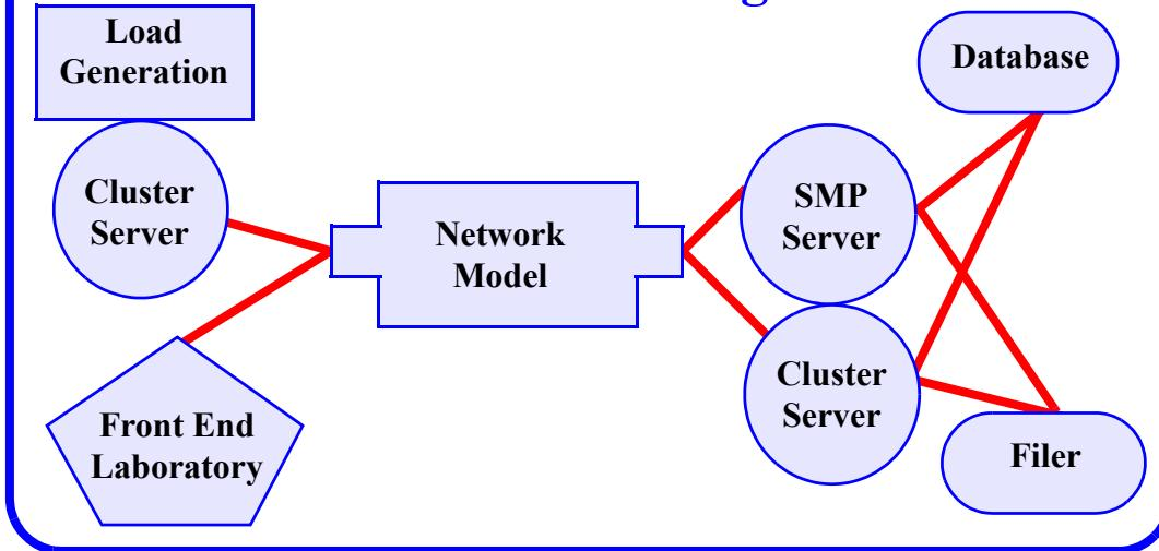
*The lab can be used for studying a typical web service by using one of the clusters to generate load and then using either a cluster server or multiple SMP servers to host the application*
