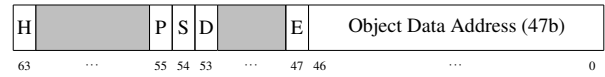
(a) Local object. H: hot, P: present, S: shared, D: dirty, E: evacuating.
