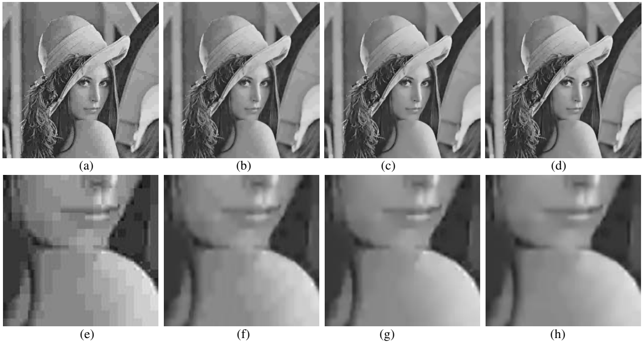
Fig. 1. Results for “Lena” (a) Coded image using Q2 (b) Robertson’s method [5] (c) Liew’s method [16] (d) The proposed method; Regions around the shoulder of “Lena”(e) Coded image using Q3 (f) Robertson’s method [5] (g) Liew’s method [16] (h) The proposed method
