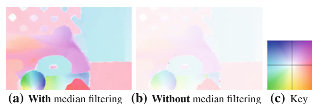
Fig. 4 Estimated flow fields on sequence “RubberWhale” using Classic-C with and without ( w/o MF ) the median filtering step. a ( w/ MF ) energy 502, 387, b ( w/o MF ) energy 449, 290, c color key (Baker et al. 2007). The median filtering step helps reach a solution free from outliers but with a higher energy. The flow fields have been normalized by their maximum magnitude resulting in different contrasts. The outliers in the result without median filtering ( b ) make the flow appear lower contrast
