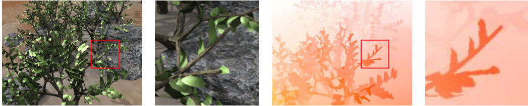
Figure 1.6. Motion boundaries: imposing smoothness across the motion boundaries will destroy the fine motion structures.
