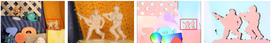
Figure 1.8. Static image information, such as color, provides strong cues to detect and preserve motion boundaries. Left pair: first frame and its enlarged detail; right pair: ground truth flow field and its enlarged detail (dark pixels correspond to occlusion regions). The motion boundaries coincide with the image edges. In addition, a pixel tends to have similar motion with pixels coming from the same surface, though the two may not be directly adjacent to each other.
