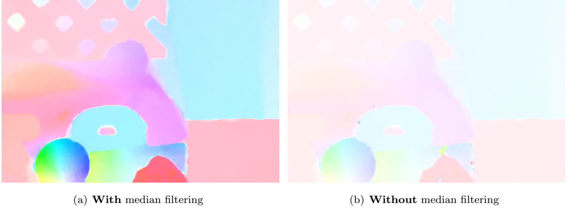
Figure 4.3. Estimated flow fields on sequence “RubberWhale” using Classic-C with and without ( w/o MF ) the median filtering step. Color coding as in [17]. (a) ( w/ MF ) energy 502,387 and (b) ( w/o MF ) energy 449,290. The median filtering step helps reach a solution free from outliers but with a higher energy.
