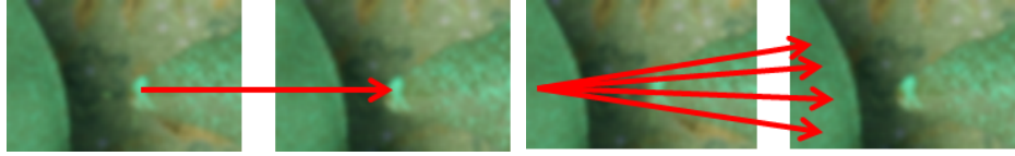
Figure 1.5. Brightness constancy is commonly assumed for optical flow estimation. It is possible to locally track salient image features (left) but not homogeneous regions (right).
