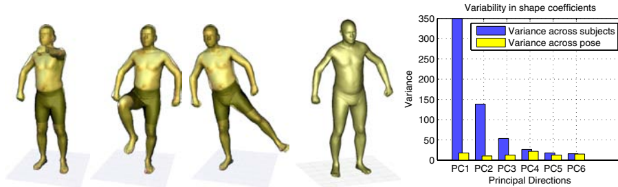
Fig. 6. Invariance of body shape to pose. (left) Reconstructions of 3D body shape for three individual poses using four camera views. (middle) Model recovered by combining across 11 different poses. (right) Variance in shape coefficients across subjects and poses.
