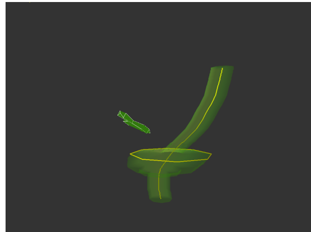
Figure 4: The width of a stroke is first modified by selecting the width attribute. This causes the stroke to become transparent, and the path, the yellow line along the length of the stroke, to be drawn. The new width of the stroke at the yellow ring is the distance between the path and the paintbrush.
