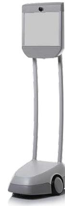
Figure 1: Beam telepresence robot, the camera and the wheels can be seen.
