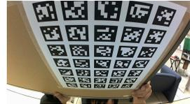
Figure 3: An optimal calibration pose suggested by AprilCal showing the tangential distortion.
