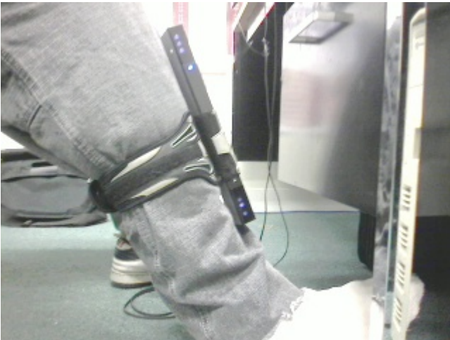
Figure 6: Players were required to wear infrared emitters attached to their legs in order for the wiimote to detect motion and gestures
