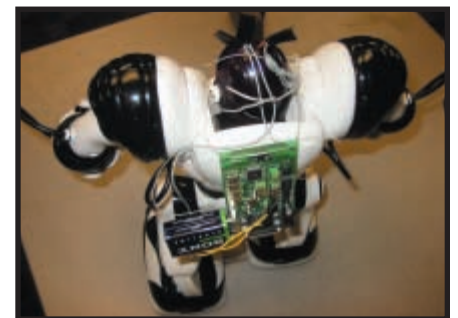
Photo 1—Check out the Robosapien 1.0. We attached a Freescale ZigBee node to its back so we could control it.
