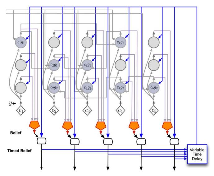
**Figure 7. Timing circuit.** The same circuit as shown in Figure 5 with the addition of circuitry for incorporating variable time delays between elements of the Markov chains. The pentagon neurons represent the belief at each node. The rounded rectangle neurons represent the belief at each node at the appropriate time delay. An external variable time delay mechanism provides time duration information to all the neurons involved in encoding sequences.
