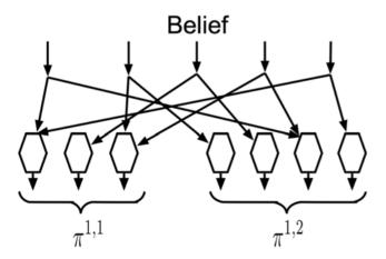
**Figure 6. Feedback message circuit.** The circuit for computing the messages to be sent to children according to Equation 9. The two sets of hexagonal neurons correspond to the Markov chains of the two children of the reference node. doi:10.1371/journal.pcbi.1000532.g006
