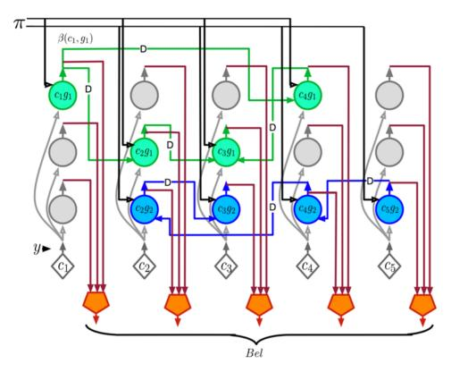
**Figure 5. Belief circuit.** Circuit for calculating the belief distribution over coincidence patterns by integrating the sequence of bottom-up inputs with the top-down inputs. The pentagon-shaped neurons are the belief neurons. These neurons pool over all the neurons representing the same coincidence in different Markov chains to calculate the belief value for each coincidence pattern. This circuit implements the Equation 6 in Table 1. doi:10.1371/journal.pcbi.1000532.g005
