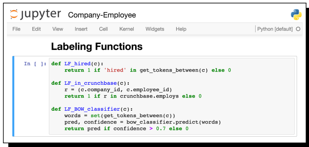
Figure 3: Labeling functions which express pattern-matching, distant supervision, and weak classifier heuristics, respectively, in Snorkel’s Jupyter notebook interface.
