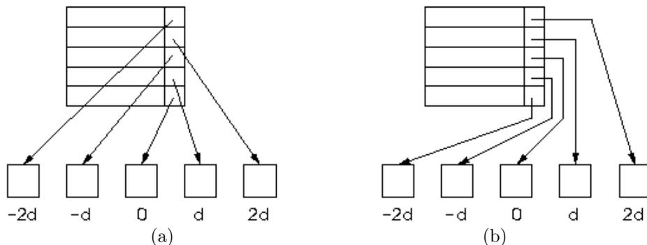
**Figure 24.2** Two strategies for assigning secondary barycenters. The value of the secondary barycenters are shown below the nodes ( $d > 0$ ). (a) Drawing with edge-node overlaps. (b) Drawing that avoids edge-node overlaps but involves additional edge routing.
