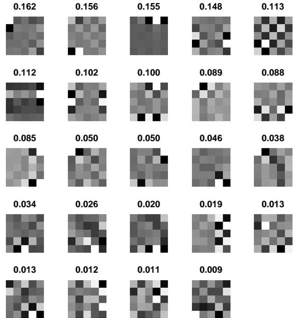
Figure 6:  $5 \times 5$  filters obtained by training the *Field-of-Experts* model with Student-t experts on a generic image database. Each filter is shown with the corresponding  $\alpha_i$ , which can be viewed as weights multiplying the log experts in the energy formulation of the model.
