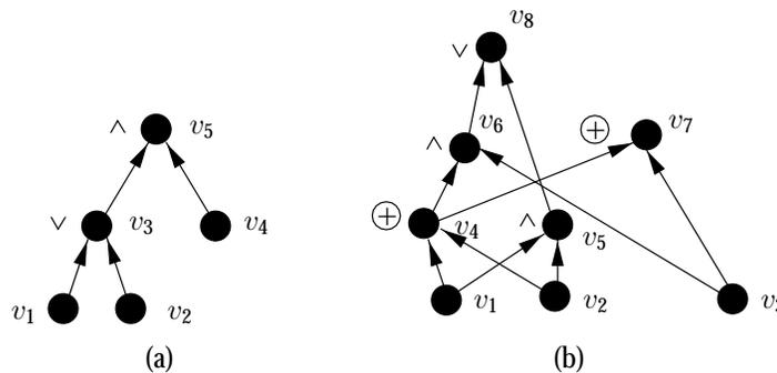
Figure 1.2 Two directed acyclic graphs representing logic circuits.
