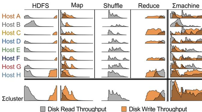
**Figure 4:** Pivot table showing disk read and write sparklines for MRsort10G. Rows group by host machine; columns group by source process. Bottom row and right column show totals, and bottom-right corner shows grand total.
