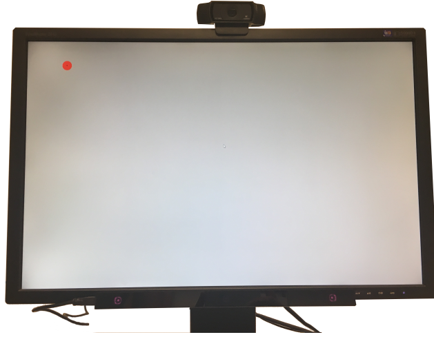
Figure 2.3: Setup of the Tobii Pro X3-120 system on the monitor of a PC. The infrared illuminators can be seen on the eye tracking bar attached to the bottom of the monitor. The screen shows a step of the calibration process, with the stimulus, which is depicted as a red circle, moving throughout the screen.
