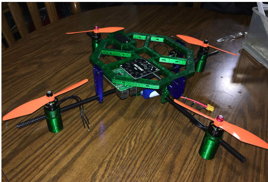
Figure 6: First prototype (missing some electronics). The far left and near right propellers tilt along the axis that connects them.
