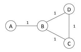
Consider network in the graph above, and only consider the routes with destination A. The network is running a distance vector protocol, and considers infinity to be 16. Use the following notation for a routing table entry: B(A,C,1) means that node B has an entry
