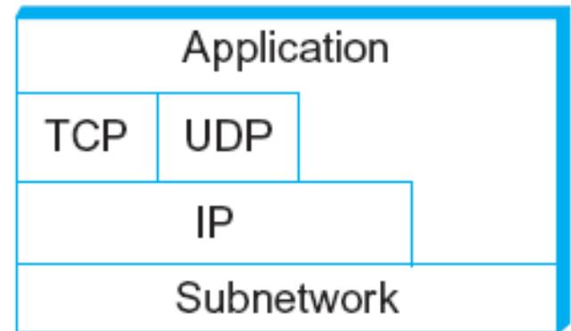
Alternative view of the Internet architecture. The “Network” layer shown here is sometimes referred to as the “sub-network” or “link” layer.
