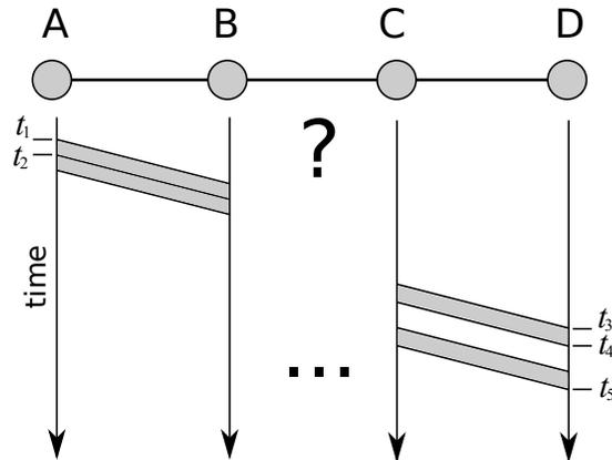
Setup: In the figure, assume there is no queueing or processing delay, and that nodes can forward a packet as soon as (a) *all* bytes for the packet have been received from the previous link, and (b) the outgoing link is free. All three links have a propagation delay of 10ms; link AB has a bandwidth of 10 Mbps ( $10^7$  bits per second), and link CD has a bandwidth of 8 Mbps ( $8 \times 10^6$  bps). You send two probe packets of 1000 bytes each, as depicted in the figure.
