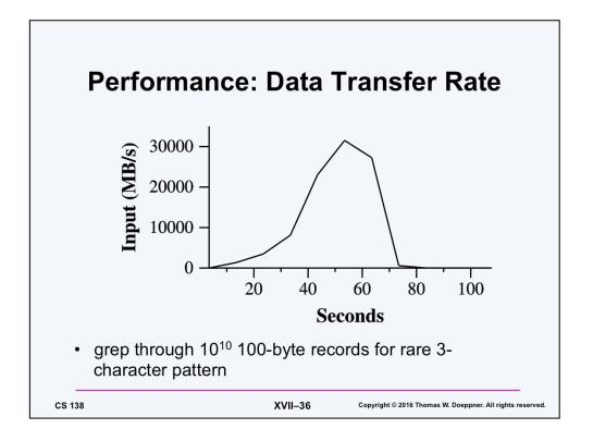
This figure is from the aforementioned paper on map reduce. 15,000 map tasks and 1 reduce task were used. 1800 computers were employed.
