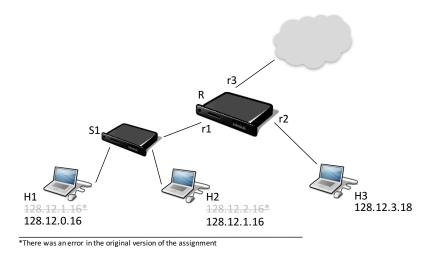
1. You are configuring this network manually. H1 and H2 are in the same subnet, and H3 is in a different subnet. What are the most specific subnet masks for H1, H2, and H3, to make this happen?
