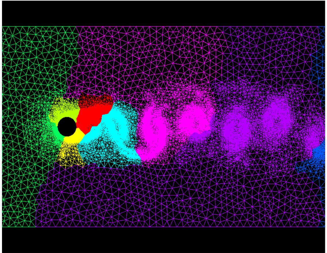
*Fig. 2 Refined mesh at time  $t = 30$  secs of incompressible fluid flow past a cylinder with Reynolds number  $Re = 250$*
